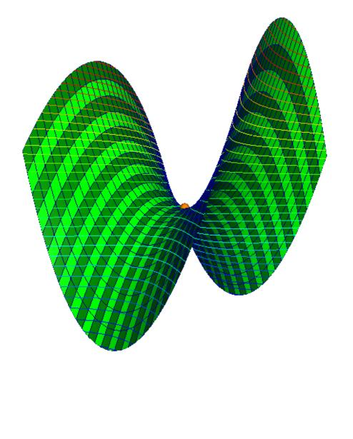
In general, z = f(x, y) may have multiple critical points and exhibit different behavior at different critical points, as in the case of function  $z = 10 - (x - 1)^2 - (y - 2)^2 + \frac{2}{81}(x - 1)^4 + \frac{2}{81}(y - 2)^4$ , whose graph is depicted below.
